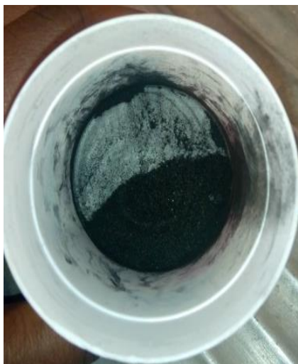
Figure 3.2: Sonication process in GO preparation and b) Graphene Oxide powder obtained after filtration and grinding
