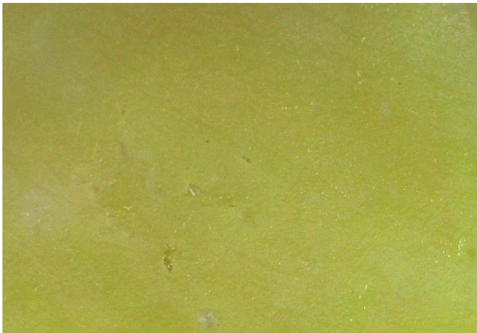
Figure 5. Microscope image of composite reinforced with 2 wt.% powder-walnut shell
