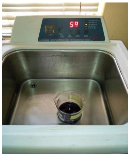
Figure 3.2: Sonication process in GO preparation and b) Graphene Oxide powder obtained after filtration and grinding
