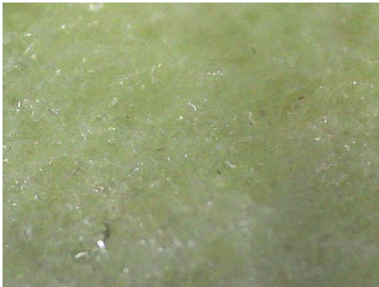
Figure 6. Microscope image of polyurethane reinforced with 1.5 wt.% organic filler
