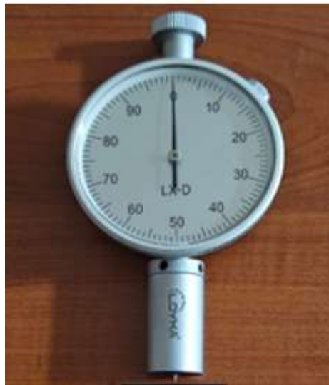
Figure 4. Shore D Durometer Used in Measurements
