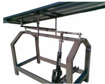
Figure 2: Solar tracker implemented practically
