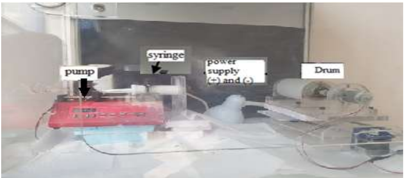
Figure 1. Electrospinning device used in nanofiber production
